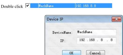
The device name can be renamed as you wish. Input IP address in controller main board panel and press OK to accept changes.
